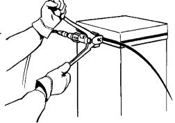
2. Bring the sealer handles completely together to assure a proper notch.
